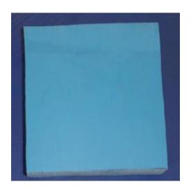
The NPL's acoustic absorber Aptflex F48 has been designed to meet the need to reduce reflections in low frequency test tanks.
