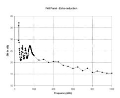
This limits or affects the performance of the tank-wall lining at high frequencies (> 1MHz).
