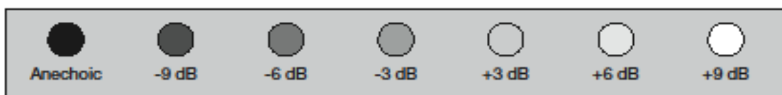
Test objects have same speed and attenuation as background
