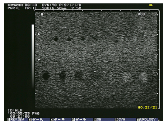
Test objects have same speed and attenuation as background
