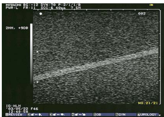
Test objects have same speed and attenuation as background
